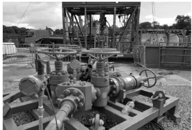
PWWT recommend a double barrier policy between process fluids and the atmosphere when changing chokes in harsh environments, such as sand clean-up and high-pressure applications. There are also variations to the adjustable choke make and type. The larger bore units and high-pressure manifolds have a production choke installed rather than the traditional needle and seat type. We can also incorporate our PowerChokes® adjustable choke, designed for severe service environments.
